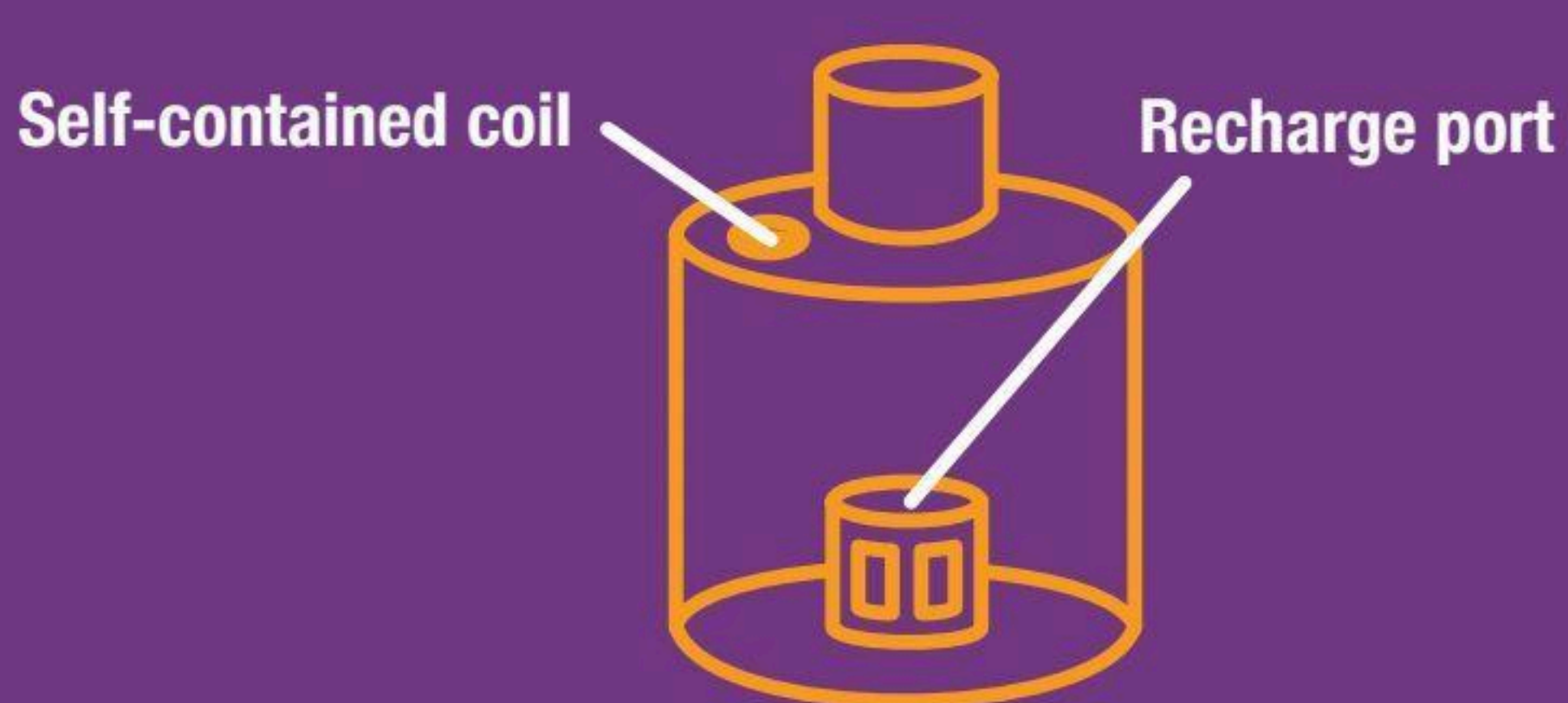
Fig 3 - A refillable tank with a replaceable coil
